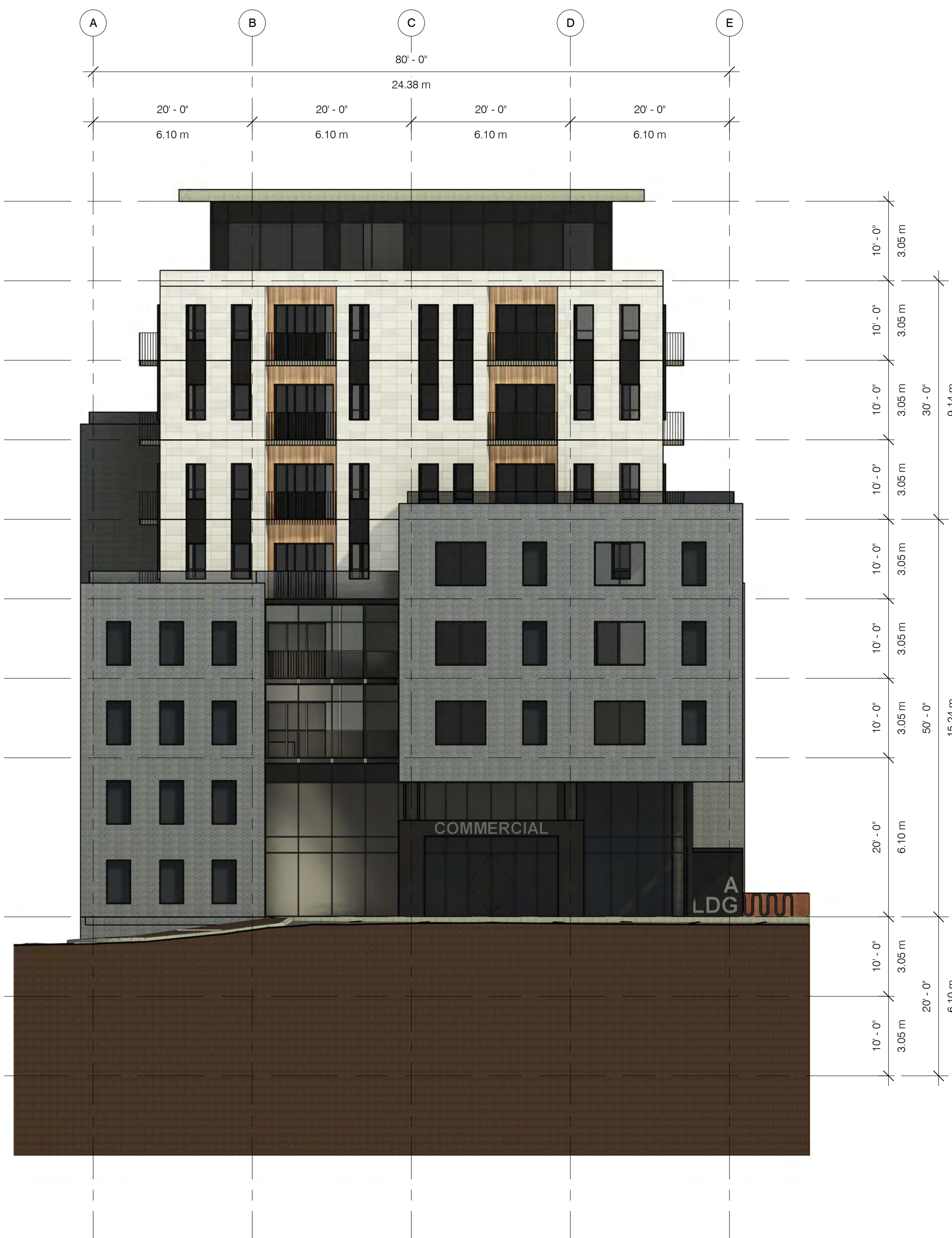
1 Building A - North Elevation A302 3/32" = 1'-0"
