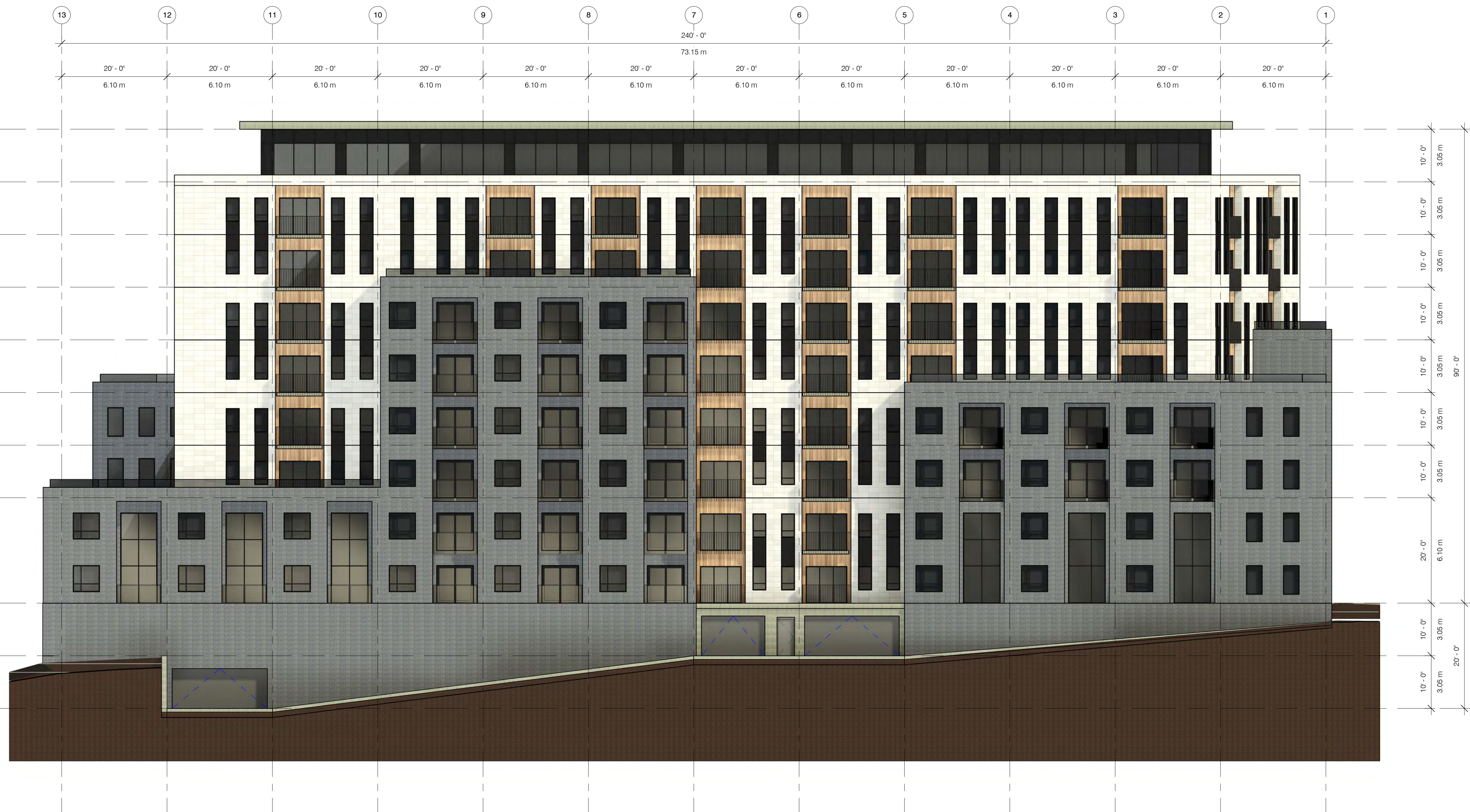
1 Building A - East Elevation A301 3/32" = 1'-0"
