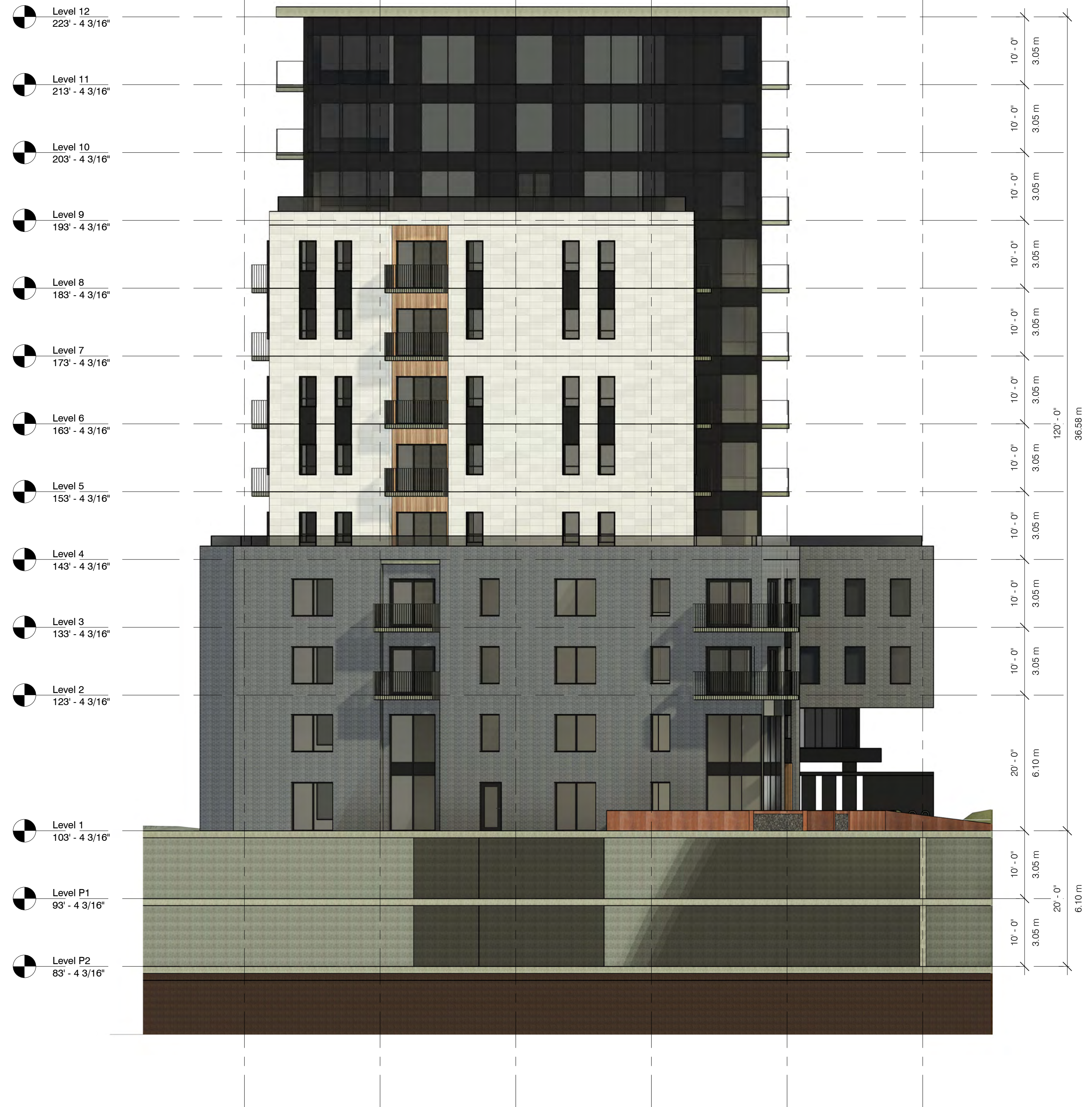
2 Building B - South Elevation 3/32" = 1'-0"
