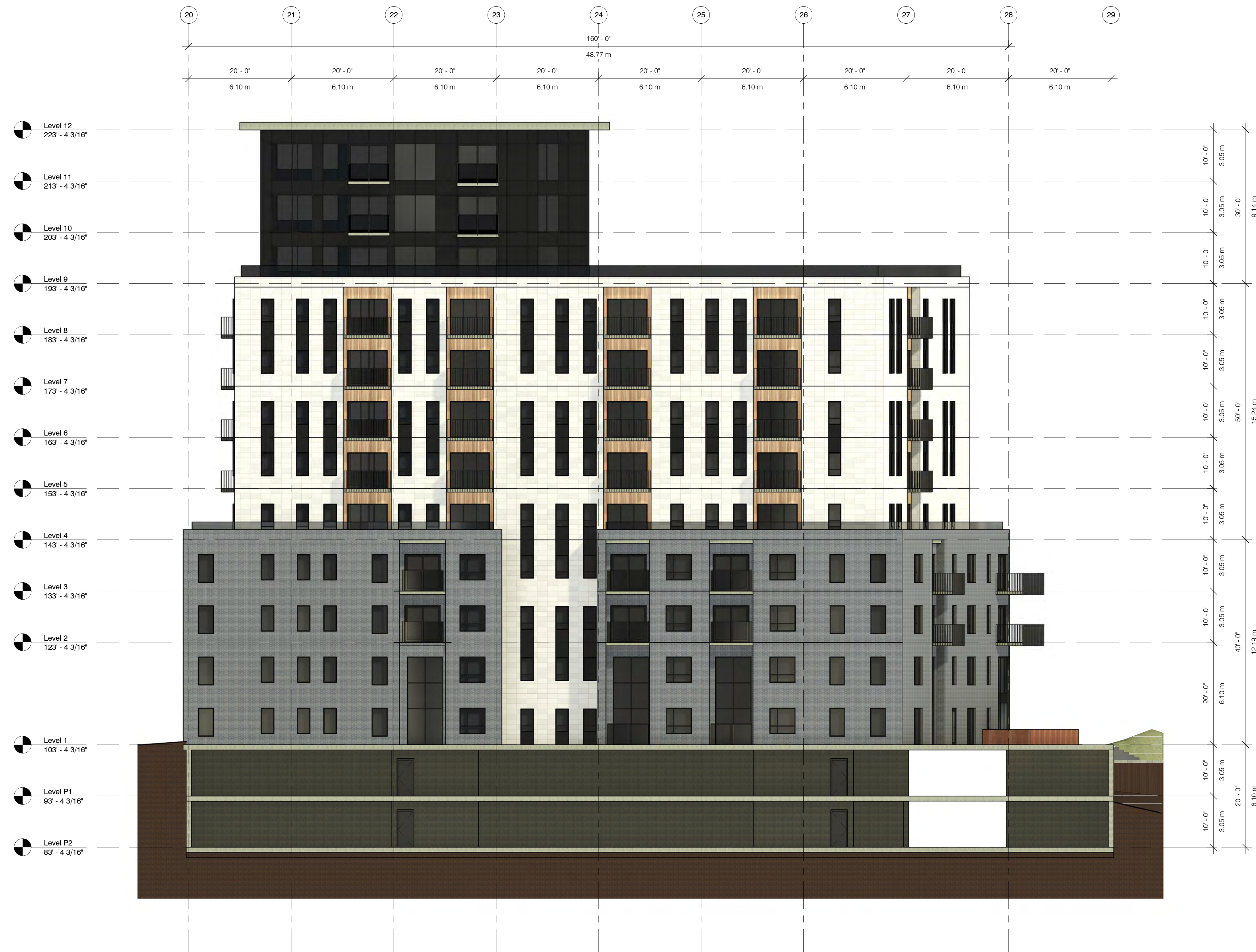
1 Building B - West Elevation A306 3/32" = 1'-0"
