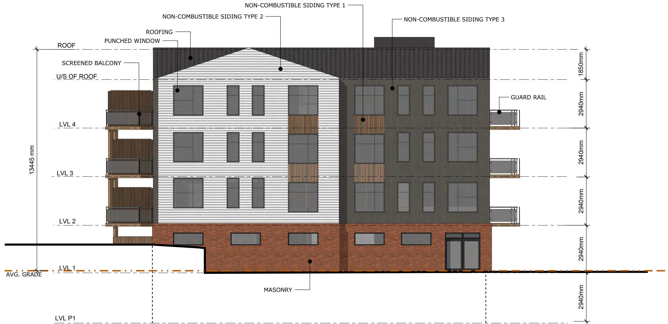
MULTI - SOUTH EAST ELEVATION
