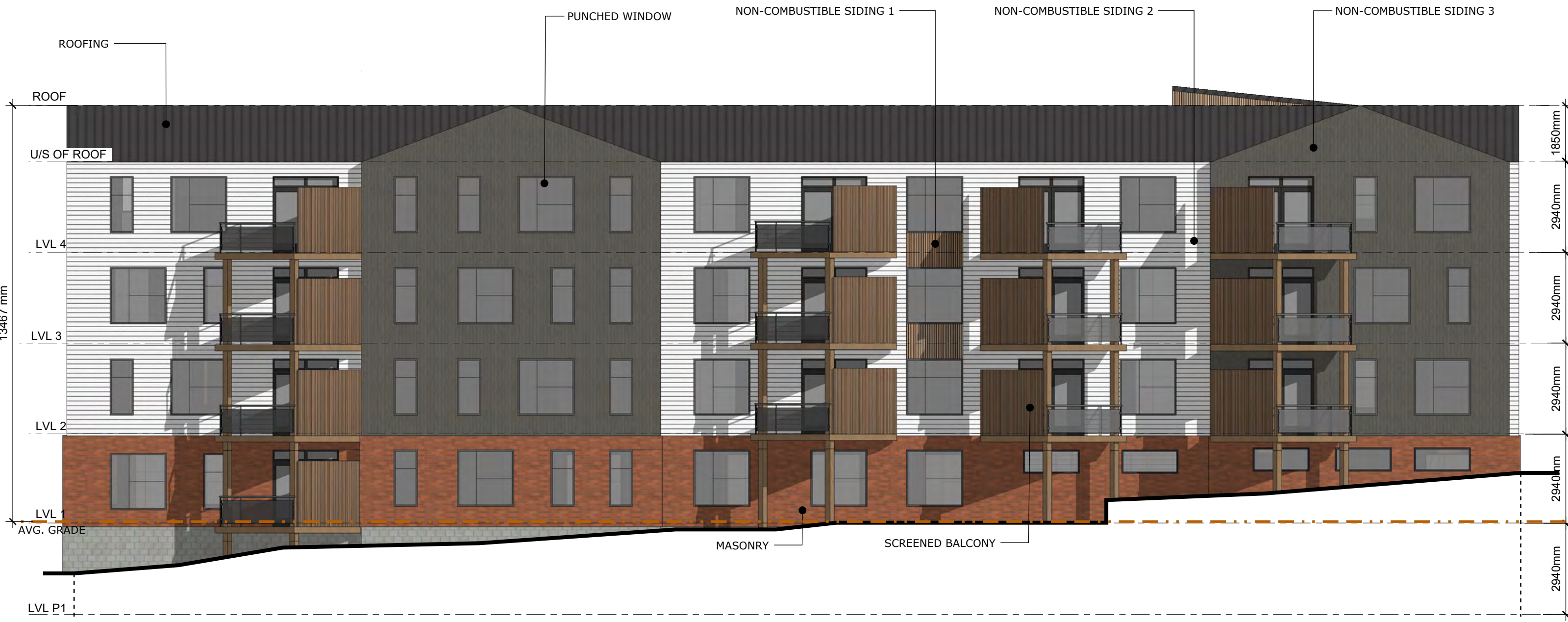
MULTI - SOUTH WEST ELEVATION
