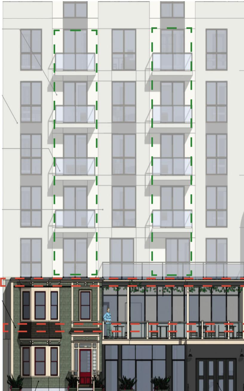
Proposed elevation with the heritage house in front of the new building. The dotted lines show the vertical and horizontal extensions of the proportion found in the Open Mic House. New parking garage entrance to right has period style doors.
