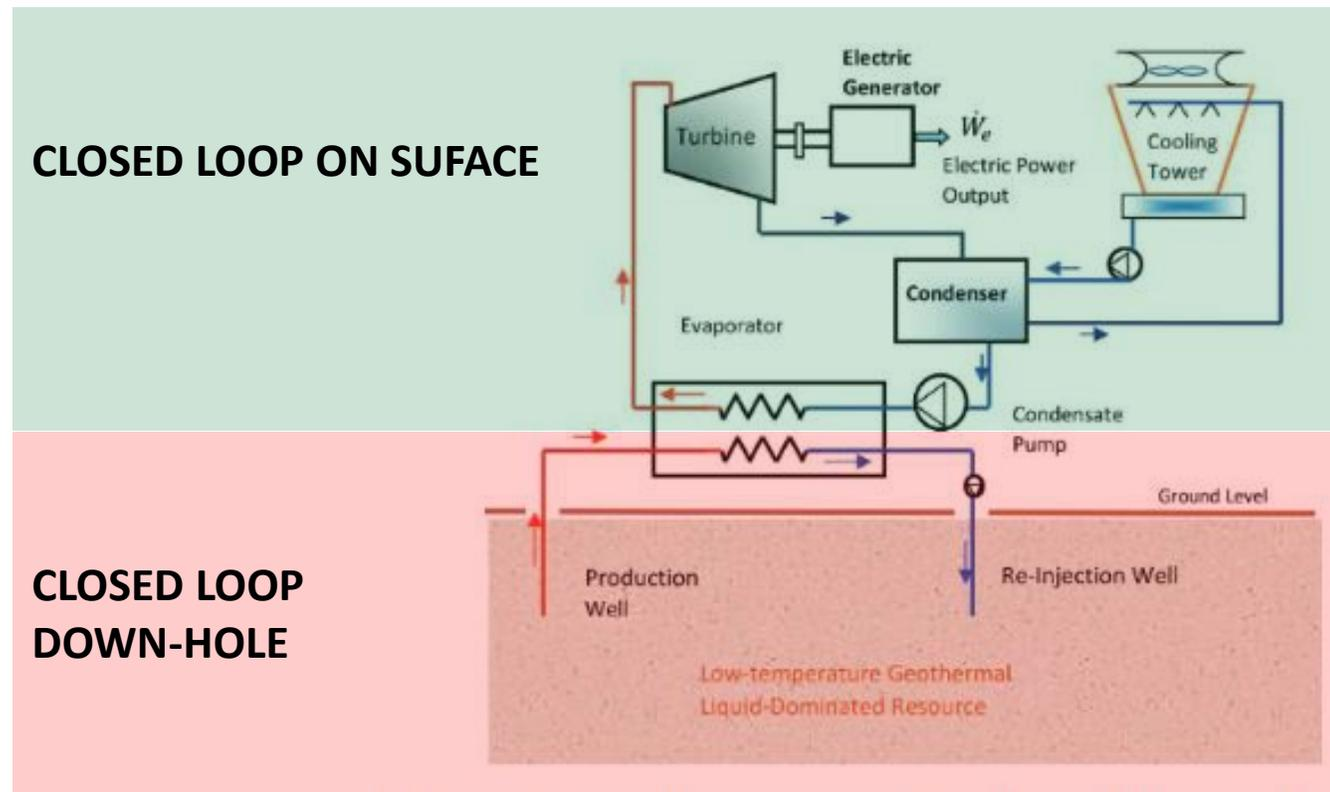
**Figure 2** Low-Temperature Geothermal Power Plant with ORC [11]
