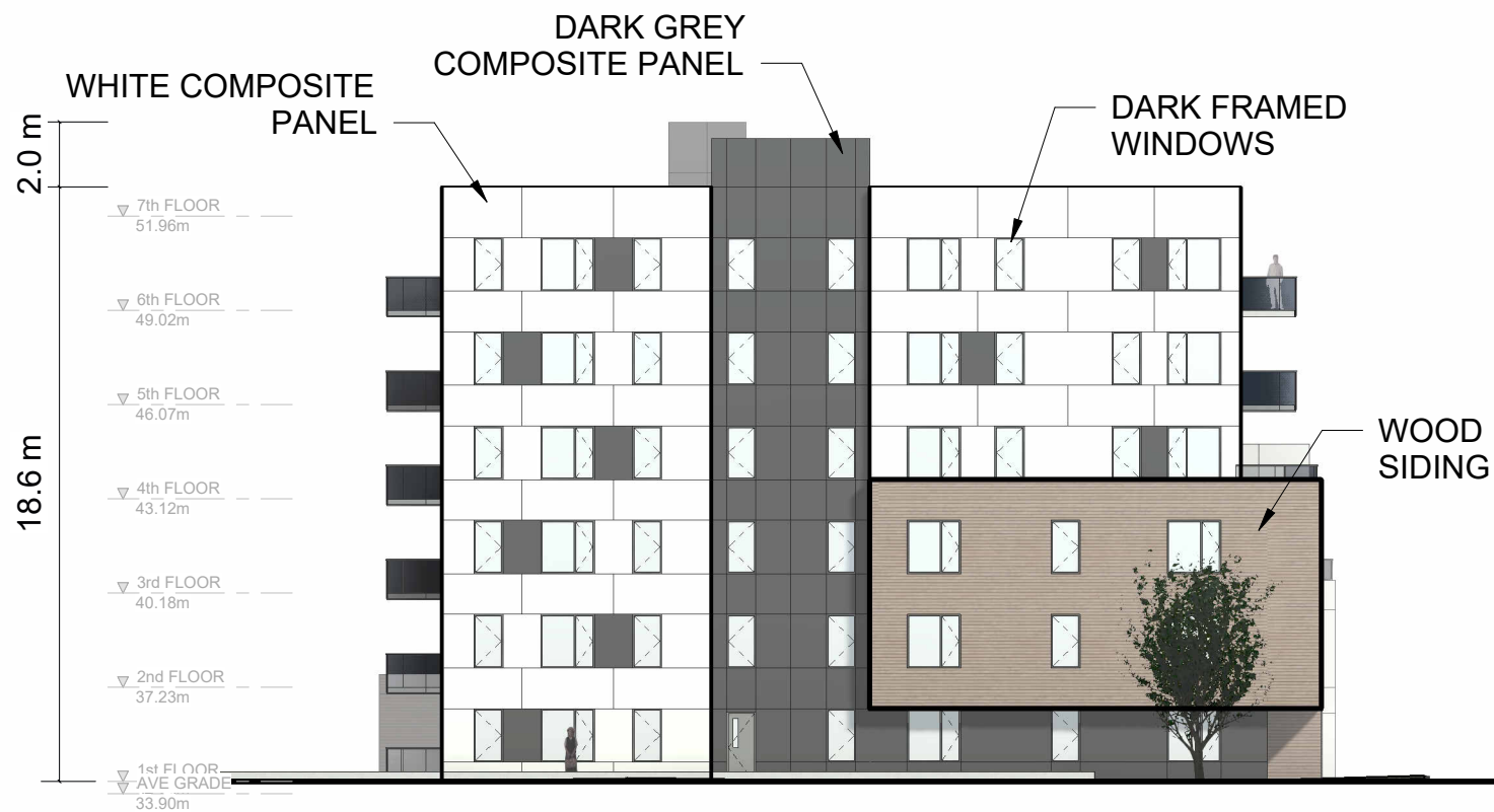
① EAST ELEVATION 1 : 240
