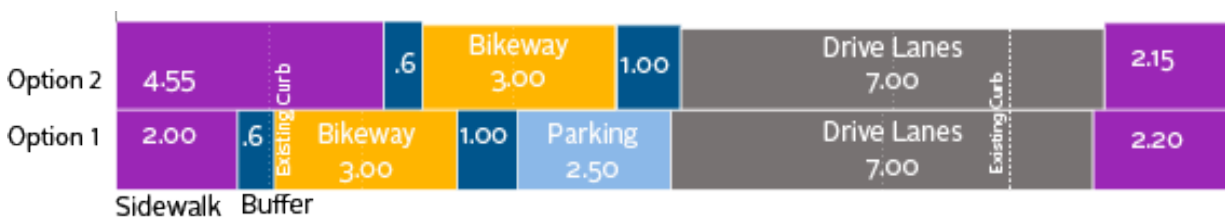
Figure 29 - Comparison of the options for the 18.3m cross section (South of Cambridge Suites Hotel to Doyle Street)
