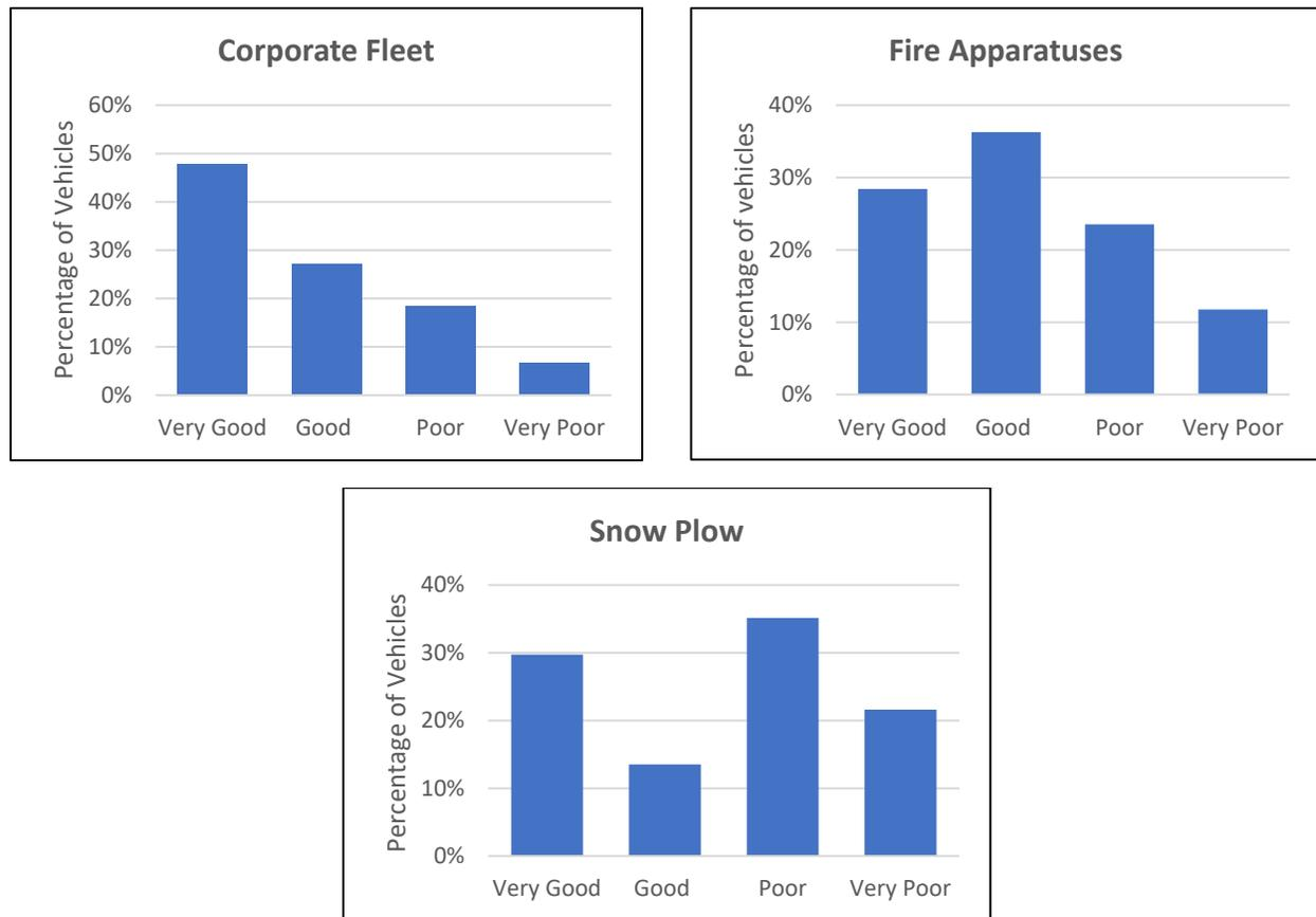
The condition ratings presented are obtained via function of the vehicle Optimal Replacement Point [ORP] score, a scoring metric used by corporate fleet staff to help visualize and schedule fleet replacement requirements in a strategic and cost-effective way. The exception to this is fire apparatuses. Their condition rating is determined by comparing the vehicles age compared to its useful life.
