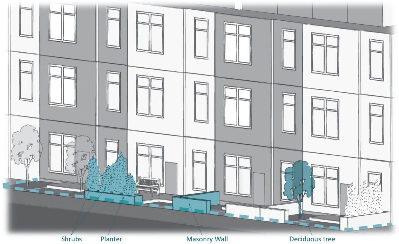
Diagram 8: Methods for providing privacy to grade-related dwelling units, per Section 151
