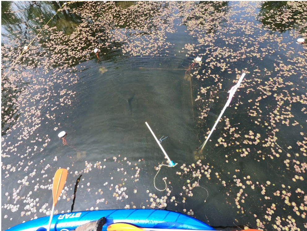
Figure 4. Overhead photo of a shallow permeable plot on May 28, 2021. Concrete blocks, horizontal rebar, and vertical marker visible under water.
