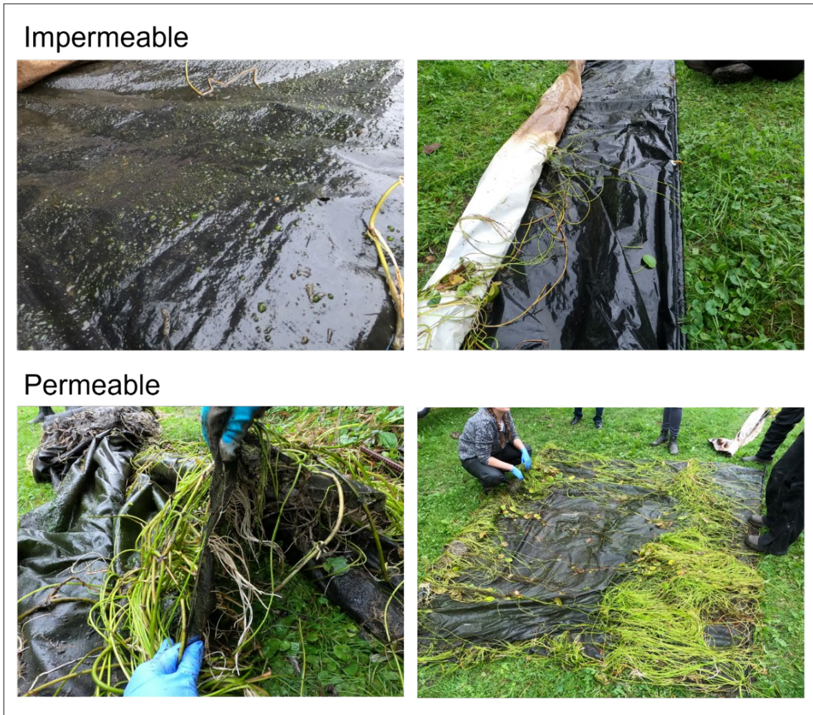
Figure 8. Barriers after removal from Little Albro Lake on September 29th, top: impermeable barrier, bottom: permeable barrier showing YFH growth through material.
