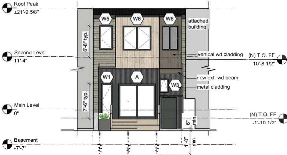
3 Proposed South Elevation 1/8" = 1'-0"
