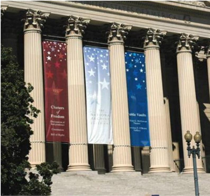
UltraMesh Eclipse is a 7.96 oz. polyester, black-backed mesh. The material is ideal for applications where complete opacity is required. UltraMesh Eclipse is UV printable and may be used for building wraps and fence graphics. Available in widths of 126 and 196 .
