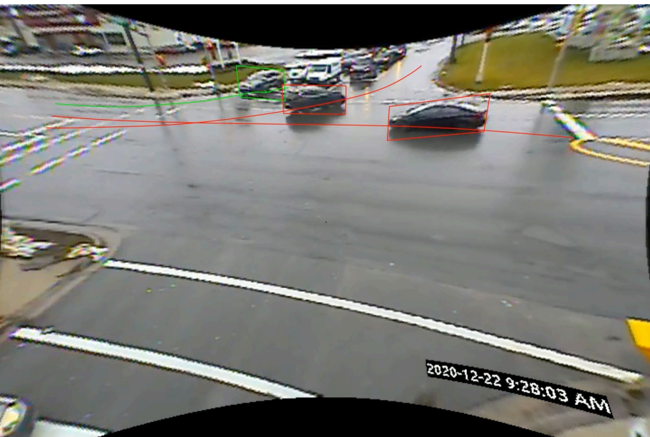
West-Left vs East-Through: PET= 1.6s, vehicle speed 56 km/h
