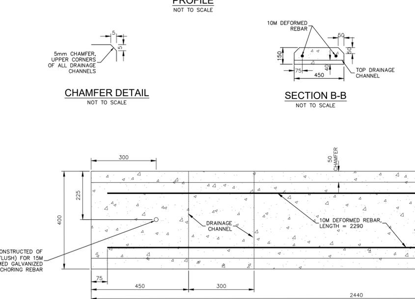
**PRE-CAST CONCRETE BIKE LANE CURB - END UNIT DETAILS**
