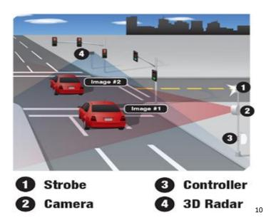
The red light camera systems used in Saskatoon, in addition to the two images, also record a 12-second digital video of the violation, which includes the six seconds prior to and the six seconds after running the red light. The captured images are sent electronically to a processing centre where vendor employees review them. If the processor identifies a violation, the images
