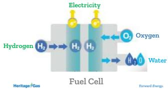
**Fuel cell vehicles ARE electric vehicles.** Batteries and fuel cells both produce electricity that can power a vehicle motor, and both can eliminate transportation emissions if zero emitting energy is used as input.
