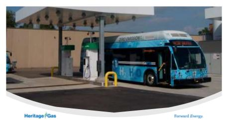
Hydrogen fuel cell electric buses can match the performance of diesel buses and are simpler to integrate into the operations of diesel bus fleets than battery electric buses. They have a range of up to 500 km. before refueling vs. 250-350
