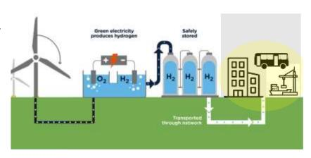
hydrogen and oxygen in a process called electrolysis. Hydrogen can be safely stored in tanks, blended with natural gas, or transported by pipe or truck to be used in other applications, like heavy transportation.
