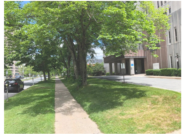
Figure 4.3.5: Appropriate Institutional Setback. Approximately 4.0 m from the streetline and comprised of vegetation but could have an improved pedestrian-oriented interface of seating and building entrances.
