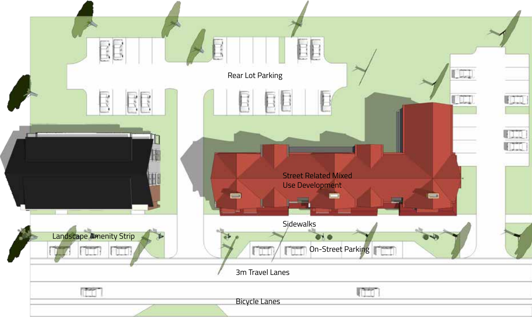
FIGURE 47. Marine Drive Upgrades
