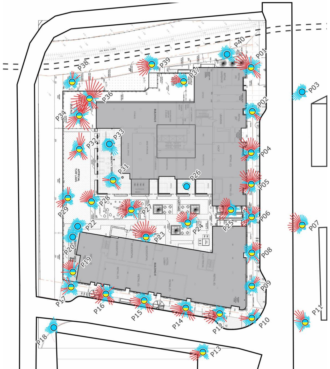
Figure 7: Wind Tunnel Results (Summer) – Parking Level 0 and Level 1 Plan Future Site Conditions (results shown without treatments applied)
