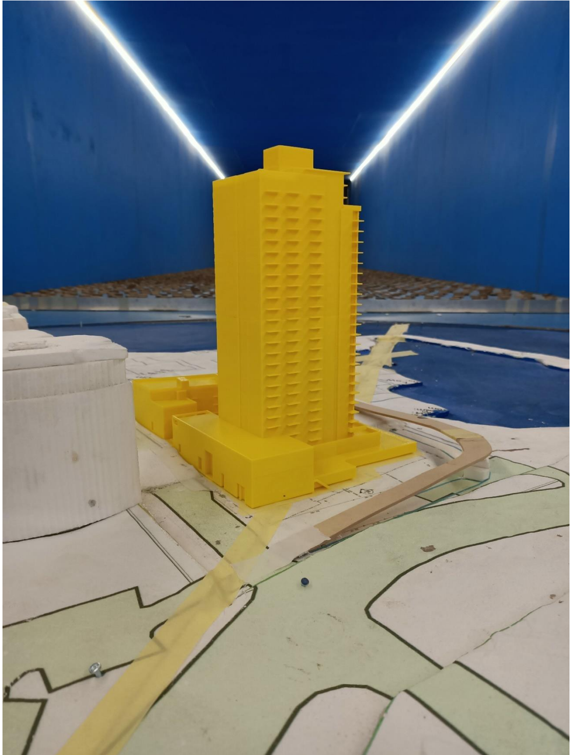
Figure 1j: Photograph of the Wind Tunnel Model – Proposed Scenario (view from the north-west)
