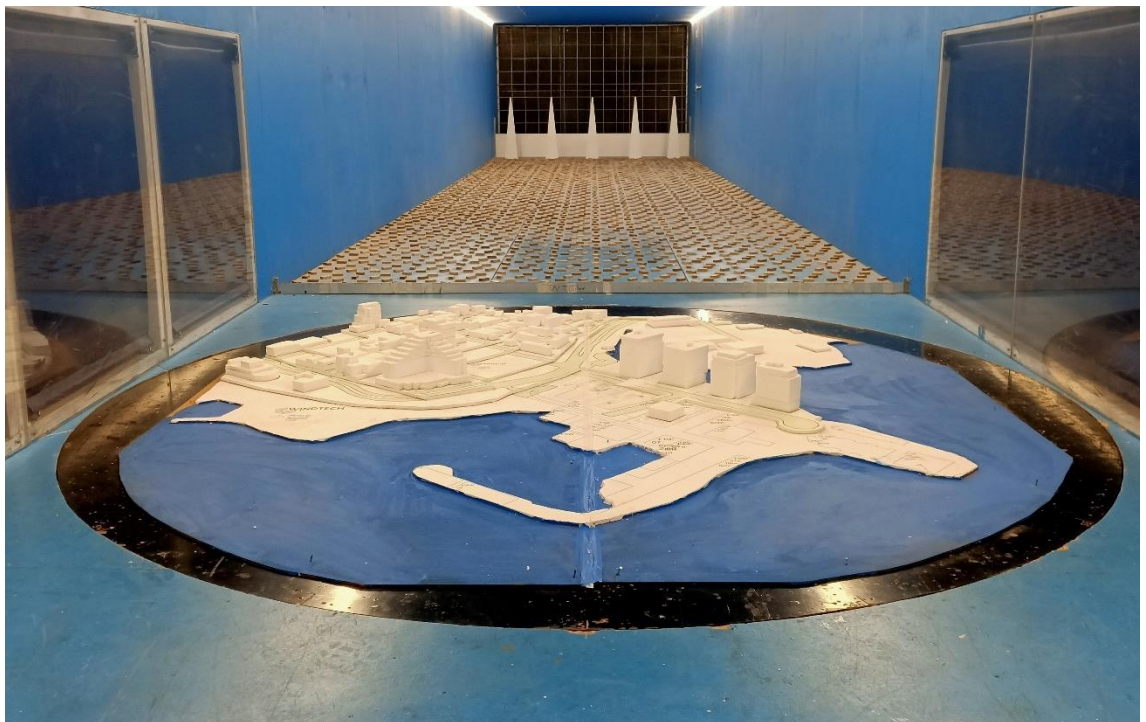
Figure 1a: Photograph of the Wind Tunnel Model – Existing Scenario (view from the south)
