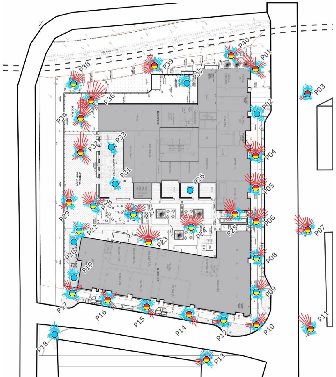
Figure9: Wind Tunnel Results (Winter) – Parking Level 0 and Level 1 Plan Future Site Conditions (results shown without treatments applied)
