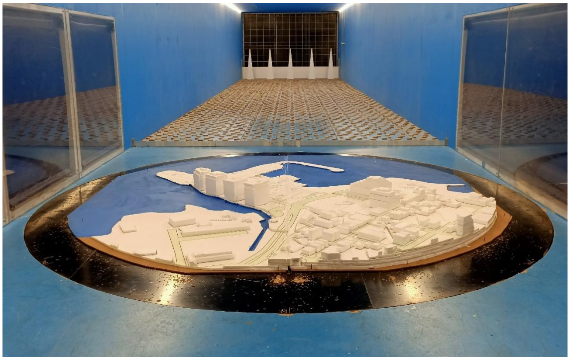
Figure 1c: Photograph of the Wind Tunnel Model – Existing Scenario (view from the north)
