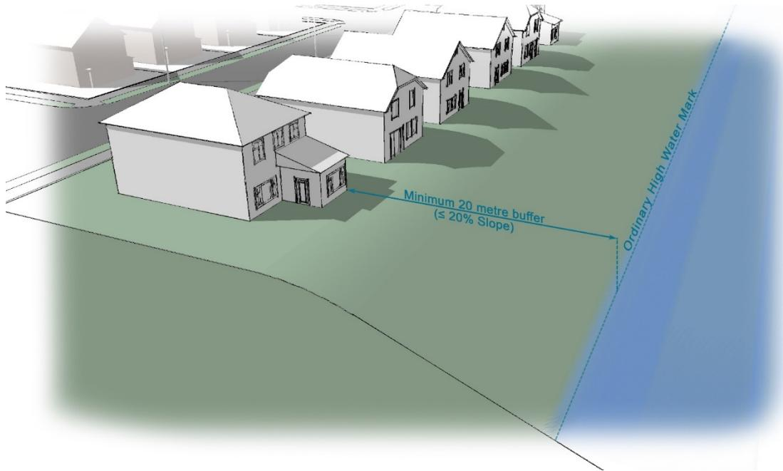
**Diagram 3:** Minimum required watercourse buffer, per Subsection 75(2)
