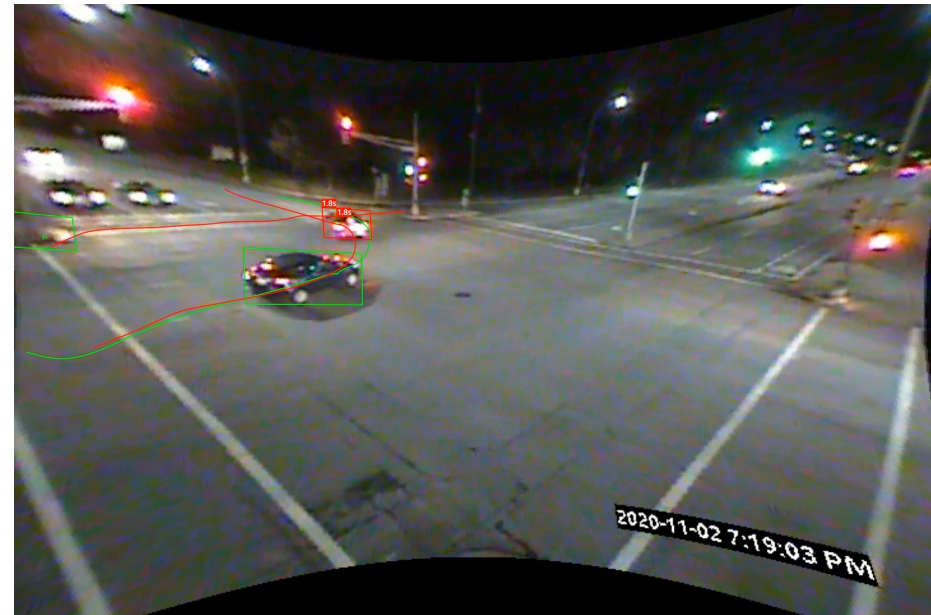
Pedestrian South Left-Hook: T2 = 1.6s, vehicle speed 20 km/h
