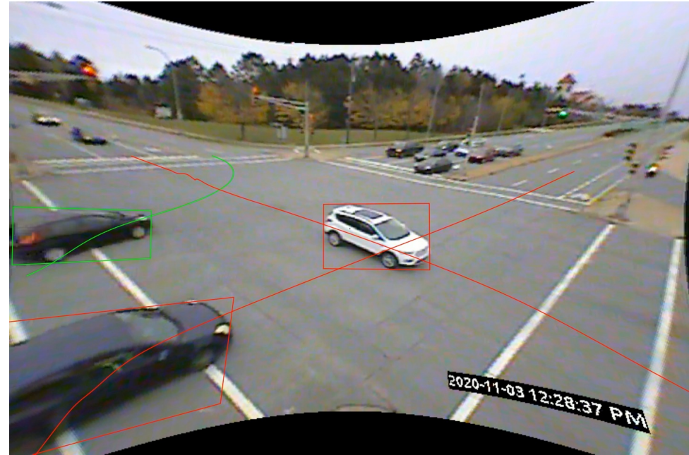
South-through vs East-through: PET = 1.8s, vehicle speed 25 km/h
