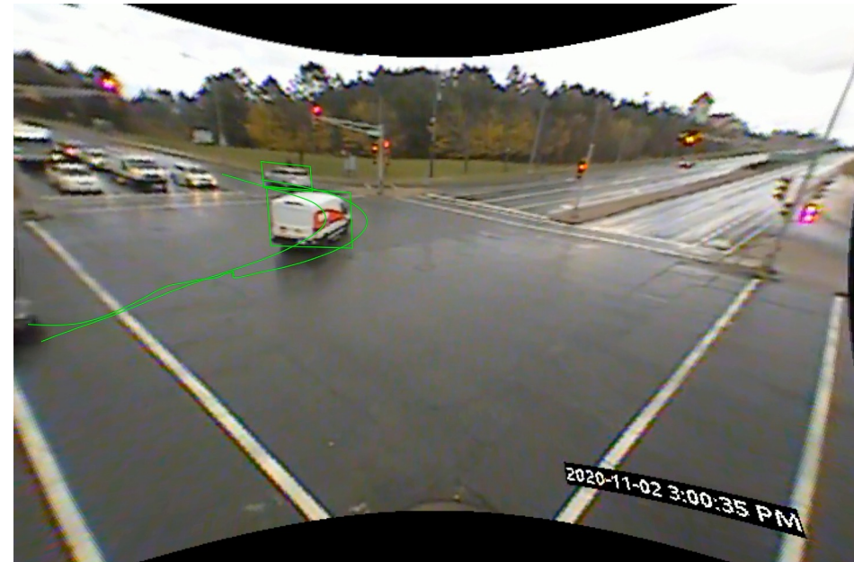
South-left vs North-through: PET = 1.2s, vehicle speed 75 km/h
