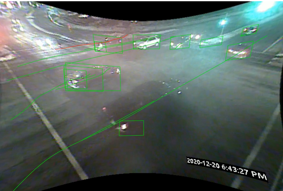
Pedestrian North Left-Hook: T2 = 2.6s, vehicle speed 14 km/h
