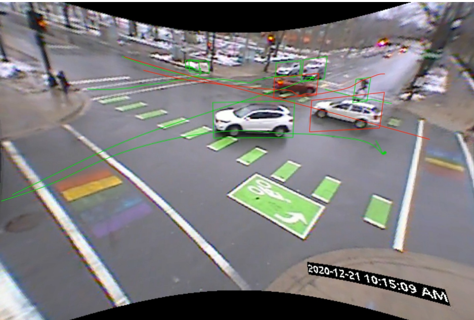
North-left vs South-through: PET = 2.3s, vehicle speed = 53km/h
