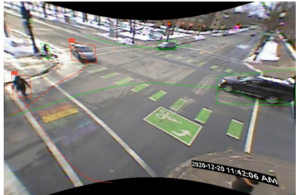
Pedestrian North-Right Hook: T_2 = 2.2s , vehicle speed = 19 km/h
