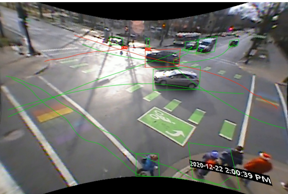
Pedestrian South-through Far-side: T_2 = 1.6s , vehicle speed = 27km/h
