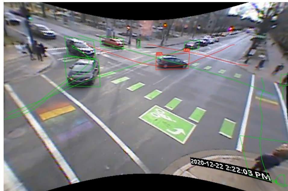
Pedestrian North-Left Hook: T_2 = 1.9s , vehicle speed = 11km/h
