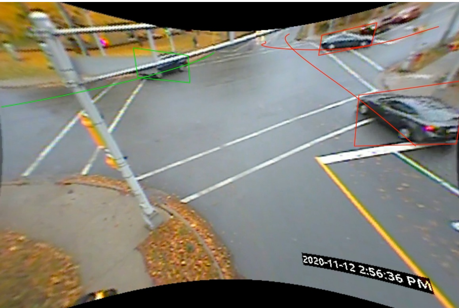
North-Left vs South-Through: PET= 2.5s, vehicle speed 42 km/h
