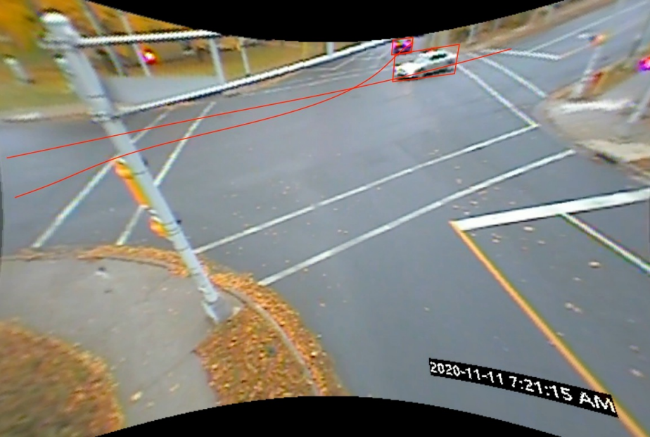
West-Left vs East-Through: PET= 2.5s, vehicle speed 55 km/h Eastbound travelling vehicles may approach the intersection with higher speeds than expected due to downgrade in topography. The skewed geometry also impacts driver sightlines as they cross the intersection. Crest curve impacts sightlines.
