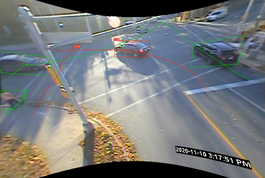
Pedestrian South-Left Hook: T_2 = 2.3s , vehicles speed = 15 km/h
