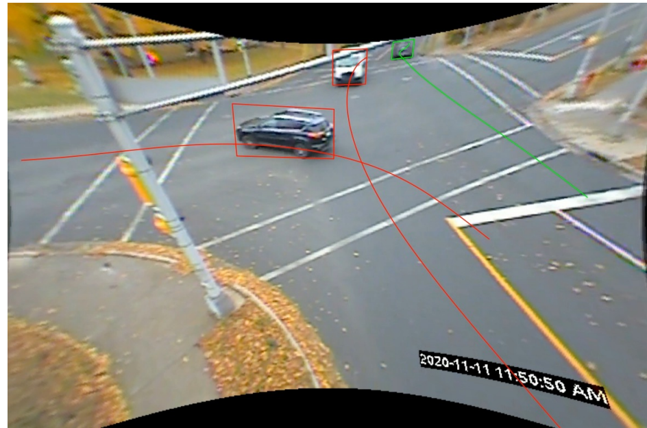
South-Left vs North-Through: PET= 1.9s, vehicle speed 52 km/h
