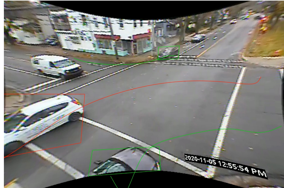
South-left vs North-through: PET = 2.0s, vehicle speed 54 km/h
