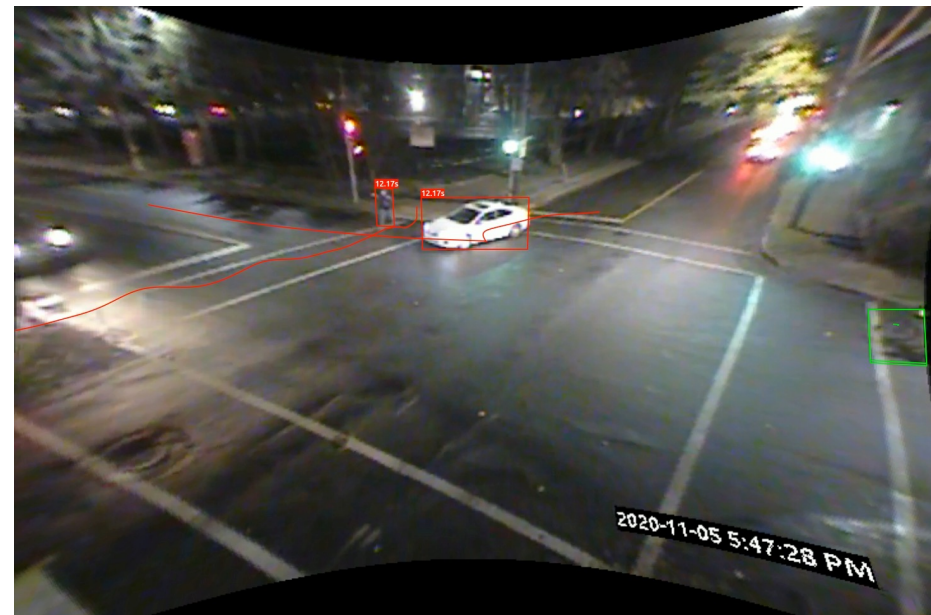
Pedestrian West Right-Hook: T_2 = 2.9s , vehicle speed 9 km/h
