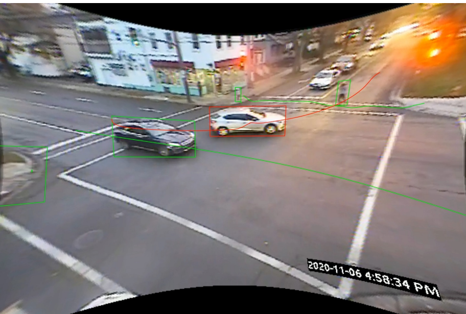
Pedestrian North Left-Hook: T_2 = 2.9s , vehicle speed 13 km/h
