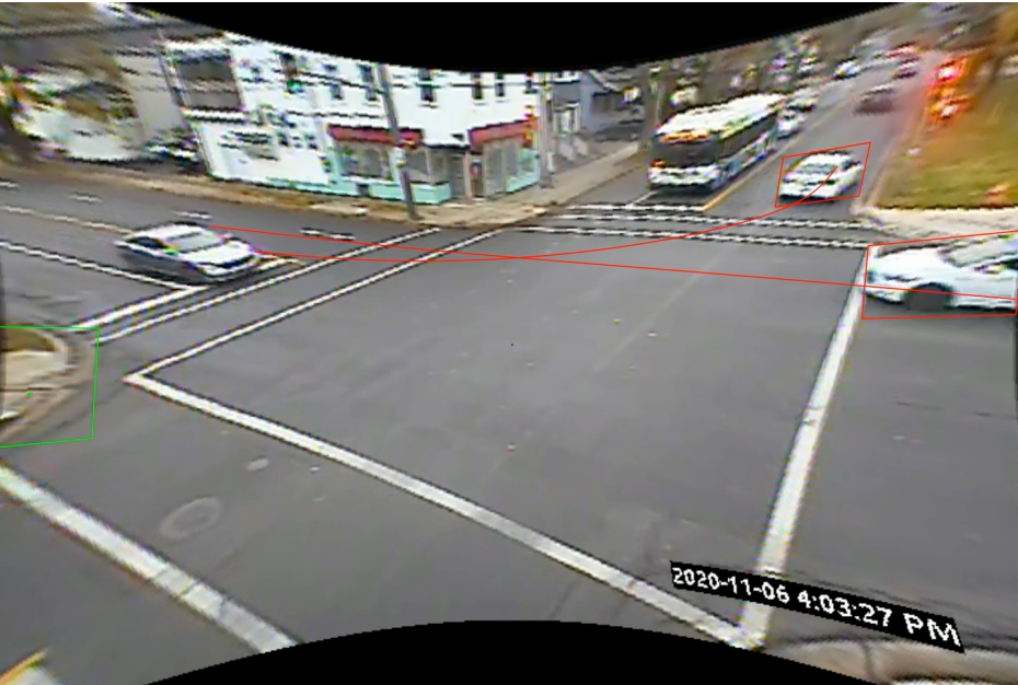
North-left vs South-through: PET = 2.5s, vehicle speed 50 km/h
