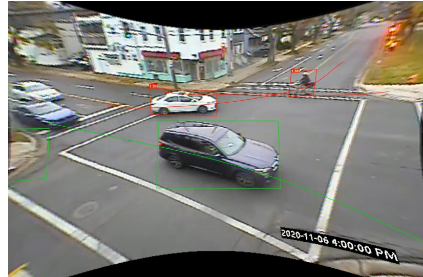
Cyclist North-Left Hook: T_2 = 1.4s , vehicle speed = 16 km/h
