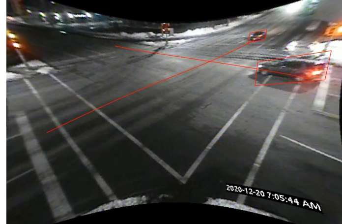
Signal Violation: south-through vs east-through
