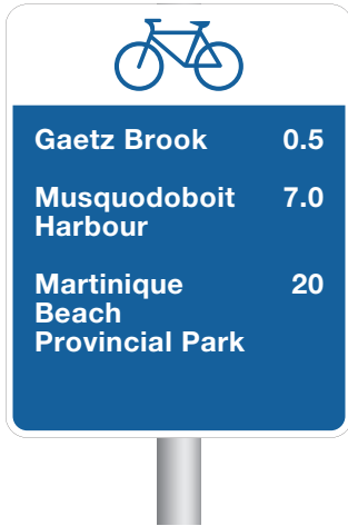
C1.1 Typical on-road confirmation sign
