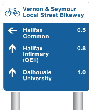
H1.2 On-road with route name When an on-road route is named, it can be shown in the header section of the sign next to the TAC bike route icon.
