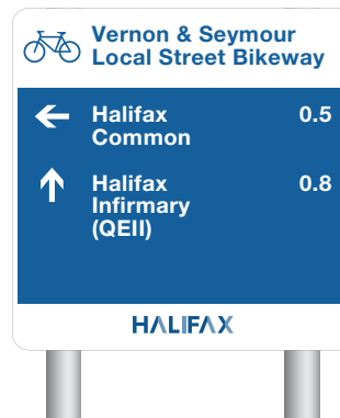
H1.3 On-road with branded footer When a route is along a municipal active transportation network, an optional footer can be used to display a brand or logo.
