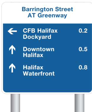
H2.1 Off-road with route name When an off-road route is named, it can be shown in the header section of the sign. If the off-road route is a bicycle only trail, a TAC bike icon can be used. If it is a multi-use trail, only the route name should be displayed.
