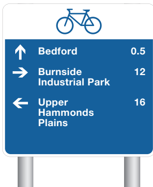
H1.1 Typical on-road hybrid sign
