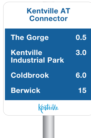
C2.3 Off-road with branded footer When a route is along a municipal active transportation network, an optional footer can be used to display a brand or logo.
