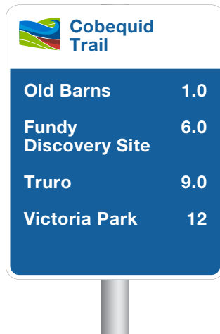
C2.2 Off-road with trail name and logo When an off-road route is named and branded, both the name and logo can be shown in the header section of the sign.
