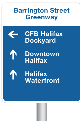
D2.1 Typical off-road decision sign Off-road routes should include the name of the trail in the header.
