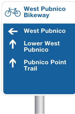
D1.2 On-road with route name When an on-road route is named, it can be shown in the header section of the sign next to the TAC bike route icon.
