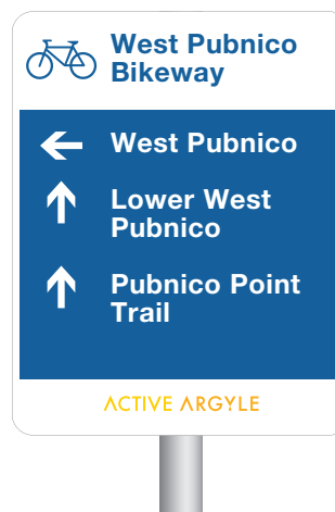
D2.3 Off-road with branded footer When a route is along a municipal active transportation network, an optional footer can be used to display a brand or logo.
