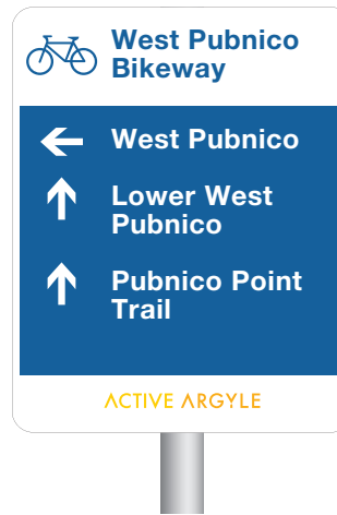
D1.3 On-road with branded footer When a route is along a municipal active transportation network, an optional footer can be used to display a brand or logo.
