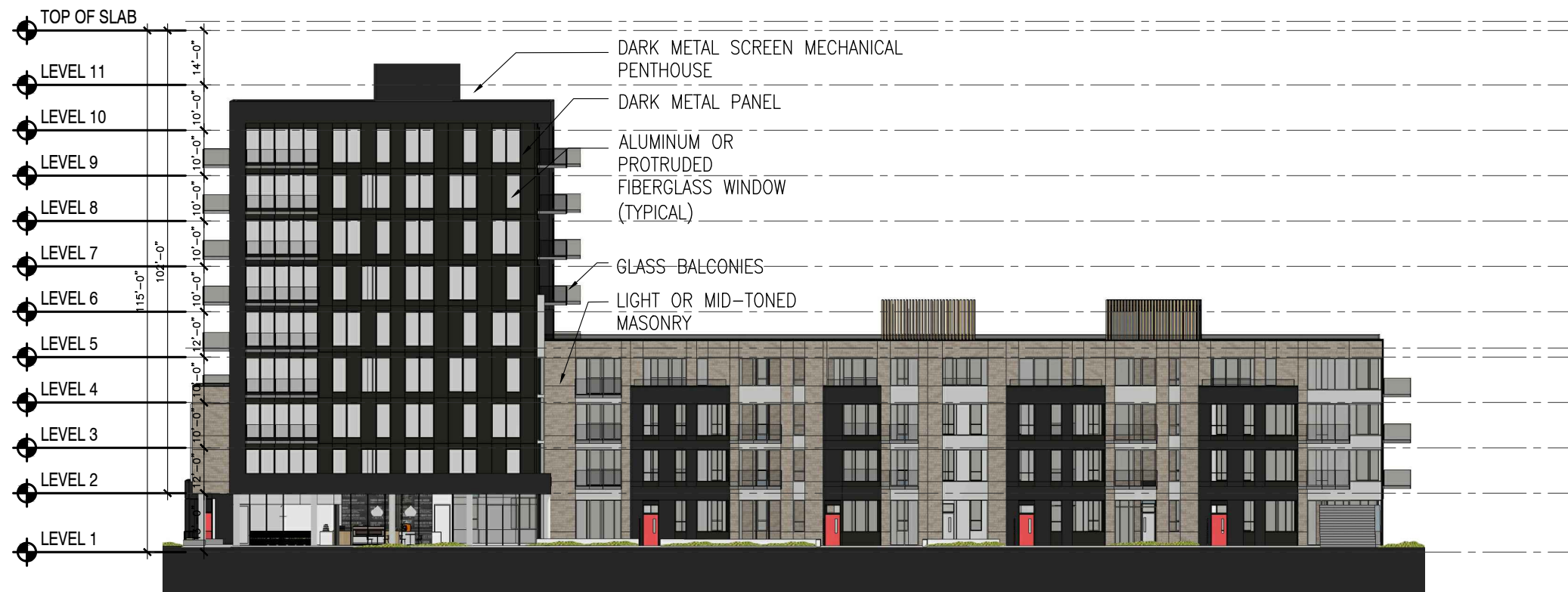
1/32"=1'-0" 1 BUILDING A- COURTYARD ELEVATION A-204
