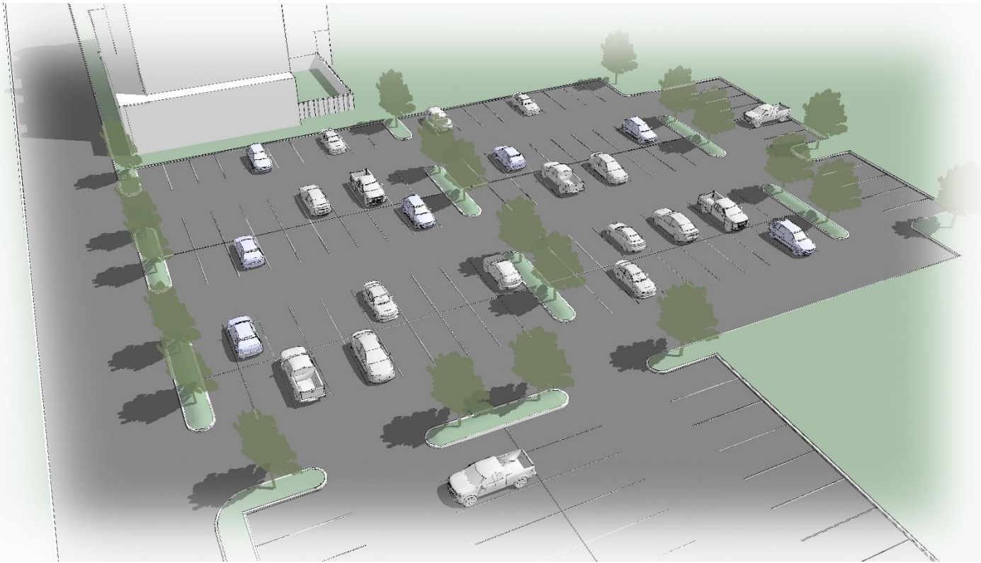
Diagram 22: Raised landscaped areas within accessory parking lots, per Subsection 427(2)
