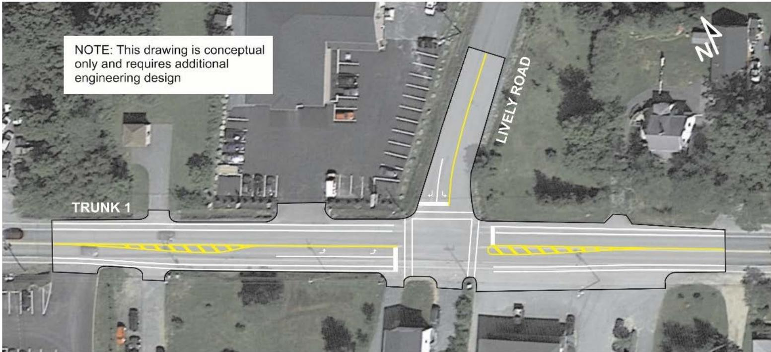
**Figure 2: Conceptual Layout of Lively/Trunk 1 Intersection**
