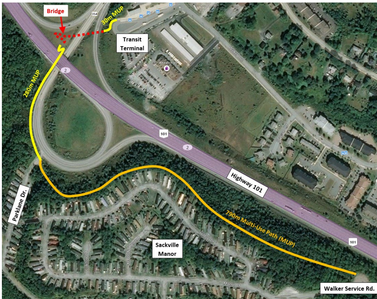
Figure 3: Option 2 proposed multi-use pathway at Beaver Bank Connector and Highway 101 Off-ramp (Exit 2)
