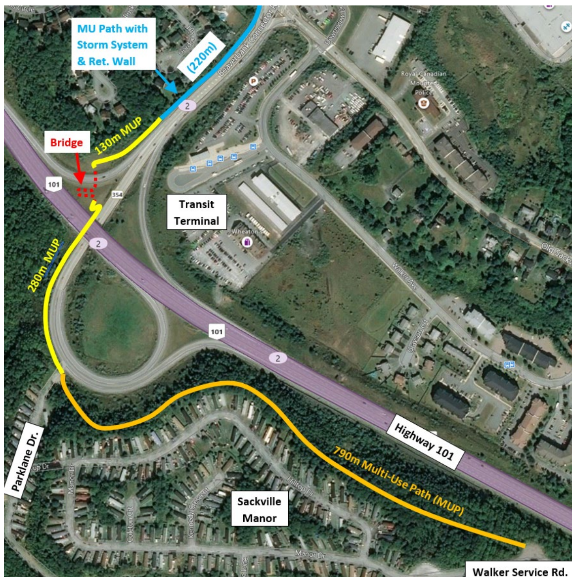
Figure 2: Option 1 proposed multi-use pathway at Beaver Bank Connector and Highway 101 Off-ramp (Exit 2)
