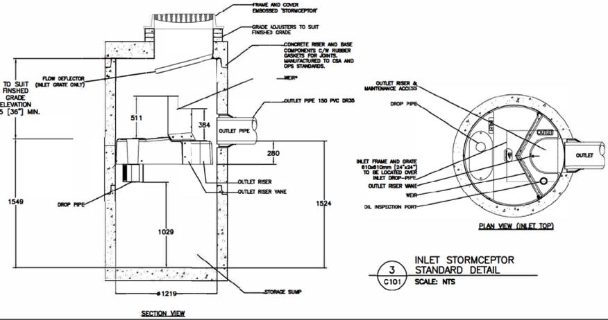
3 INLET STORMCEPTOR STANDARD DETAIL SCALE: NTS
