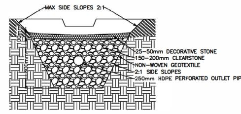
1 ROCK TRENCH CROSS SECTION SCALE: NTS
