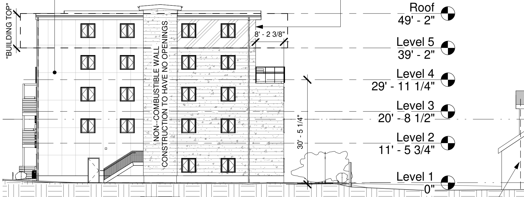
① Elevation - Side (1) (Small Scale) 1/16" = 1'-0"
