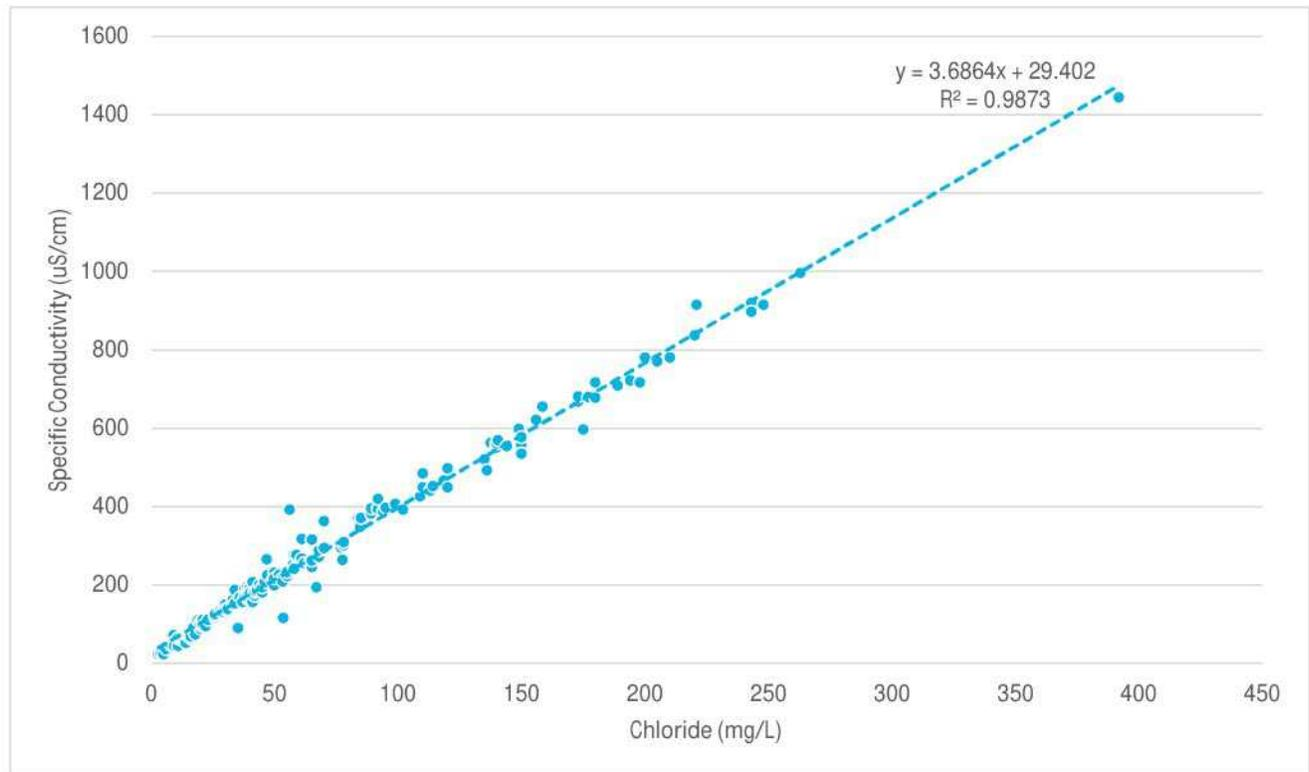
**Figure 10: Relationship between Chloride Concentration and Specific Conductivity in HRM Lakes**
