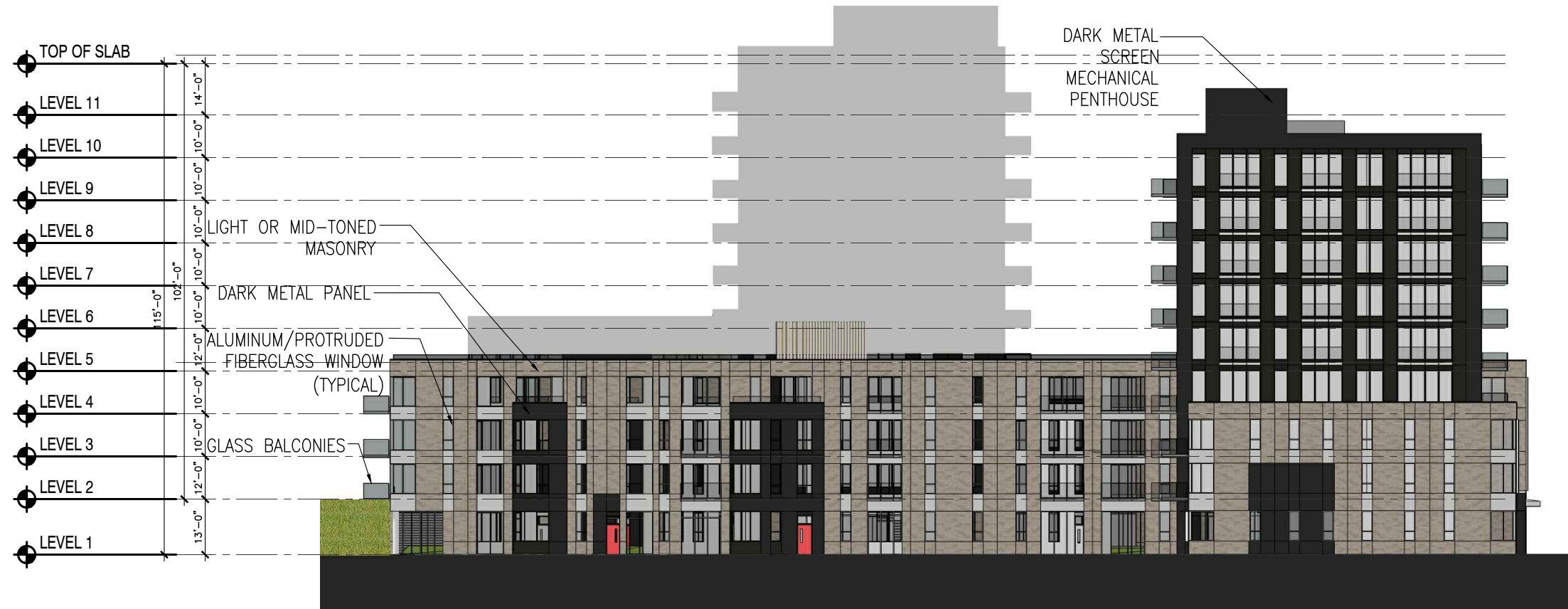
1/32"=1'-0" 1 BUILDING A- FRASER ST ELEVATION A-202
