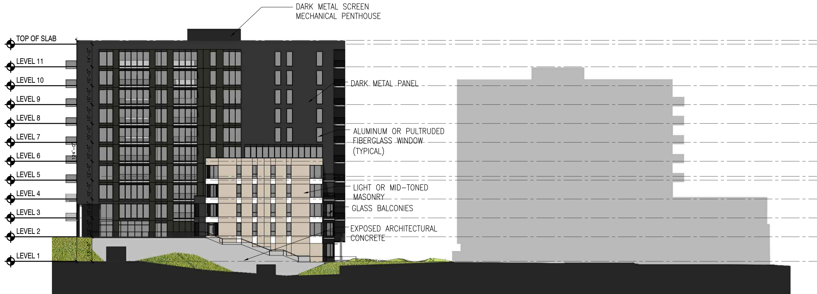
1/32"=1'-0" 1 BUILDING B- HESTER ST ELEVATION B-201
