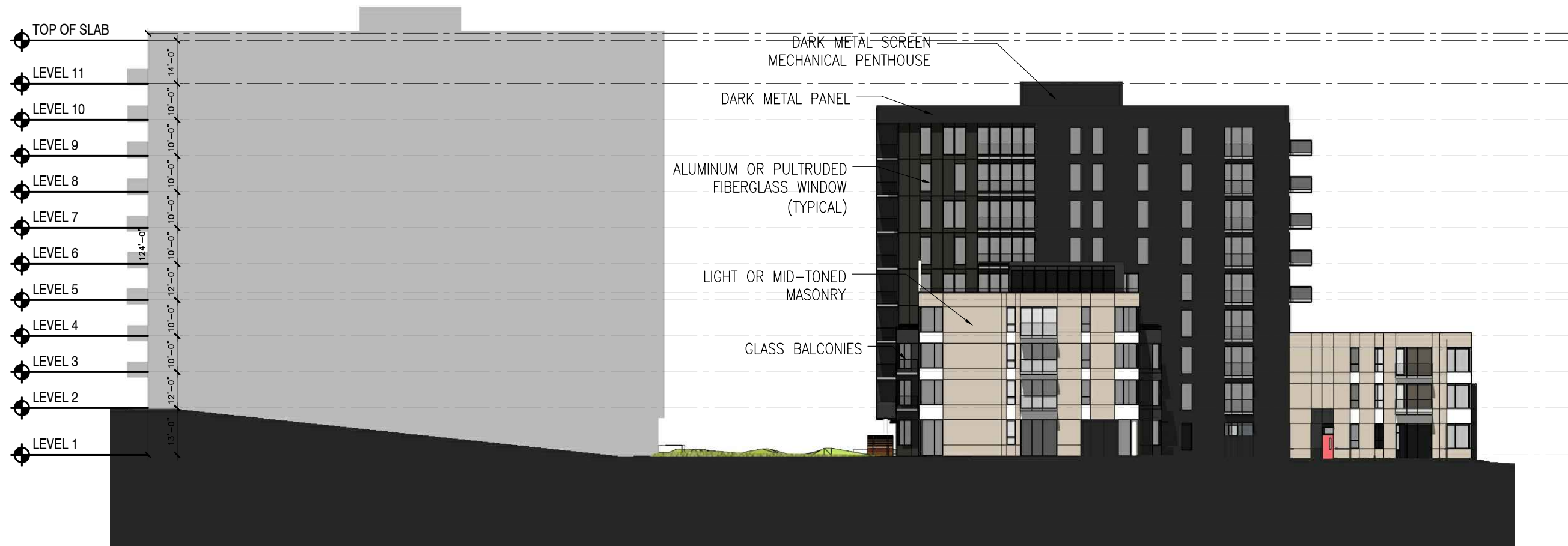
1/32"=1'-0" 1 BUILDING A- HESTER ST ELEVATION A-201
