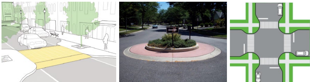
From left to right: Figure 4: Sample image of a vertical deflection (speed table); Figure 5: Sample image of a mini traffic circle; Figure 6: Sample image of curb extensions aka bump outs
