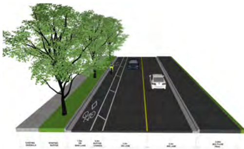
Almon Street looking Eastward: Protected Bicycle Facility through Connaught Avenue Pinch Point
