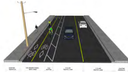
Option 2: Cornwallis Street Two-Way Protected Bicycle Facility
