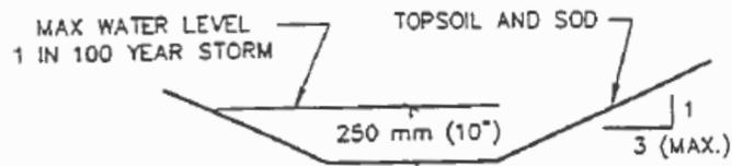
FIGURE 1b: SWALE AND UNDERDRAIN CROSS SECTION
