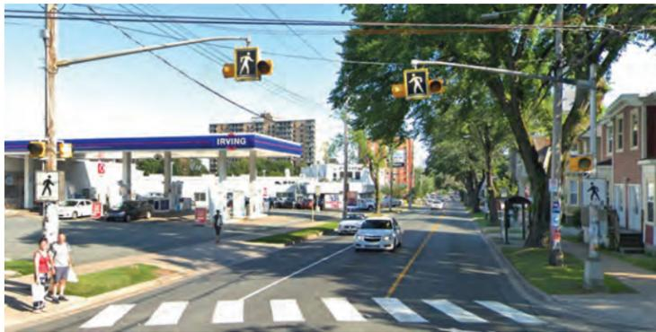
Overhead Flashing Beacons pedestrian crossings control the flow of traffic with the use of a pedestrian push-button or cyclist sensor that activate flashing lights above the road.
