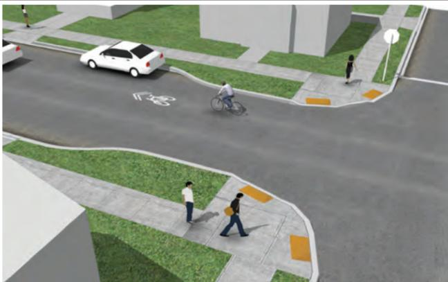
Curb extensions are a traffic calming measure primarily used to extend the sidewalk, reducing the crossing distance and providing better visibility of the pedestrian.
