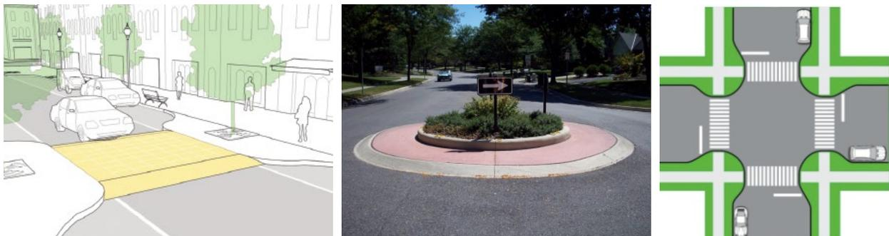
*From left to right: Figure 4: Sample image of a vertical deflection (speed table); Figure 5: Sample image of a mini traffic circle; Figure 6: Sample image of curb extensions aka bump outs*
