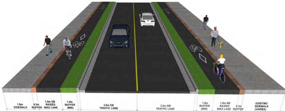
**Figure 4-7: Concept Design – Option B (Typical)**
