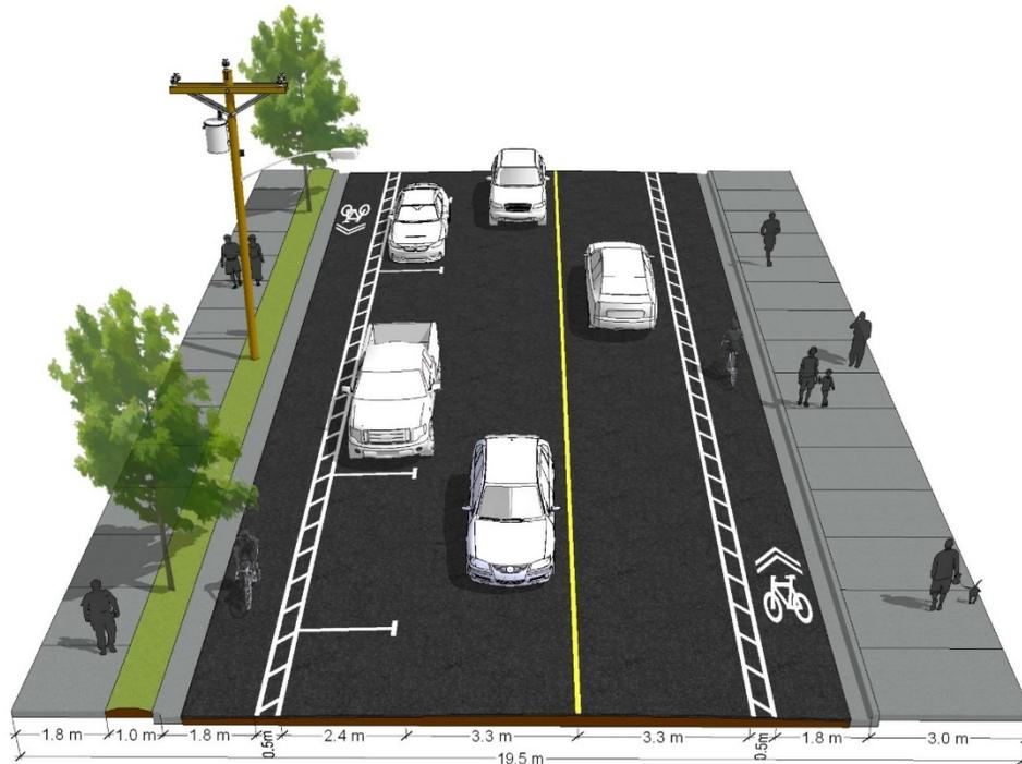
Figure 2: Cross-section of Option 1
