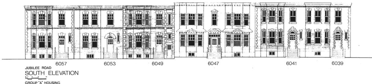
Figure 4: Edward Maxwell's rowhouse development. 6047 Jubilee Road is the only timber-frame building and it is twice as wide as the other rowhouses constructed of load-bearing brick.
