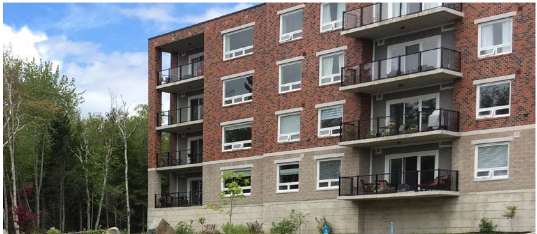
Figure 4: Multi-unit residential building with a small casement windows that are easily accessible from interior of units. First floor units are also raised above grade to improve safety and security
