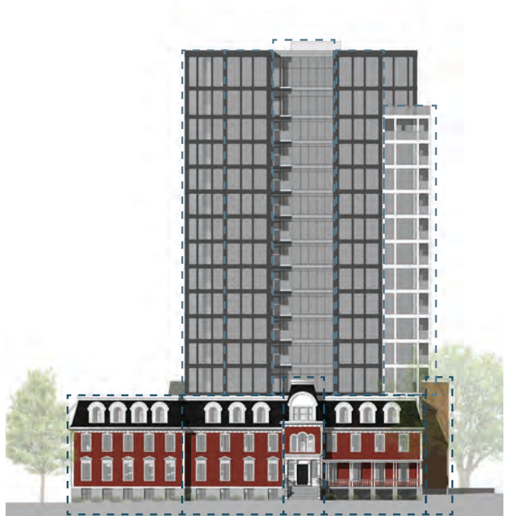
Fig. 29 Rhythm of bays along Victoria Hall and the new building
