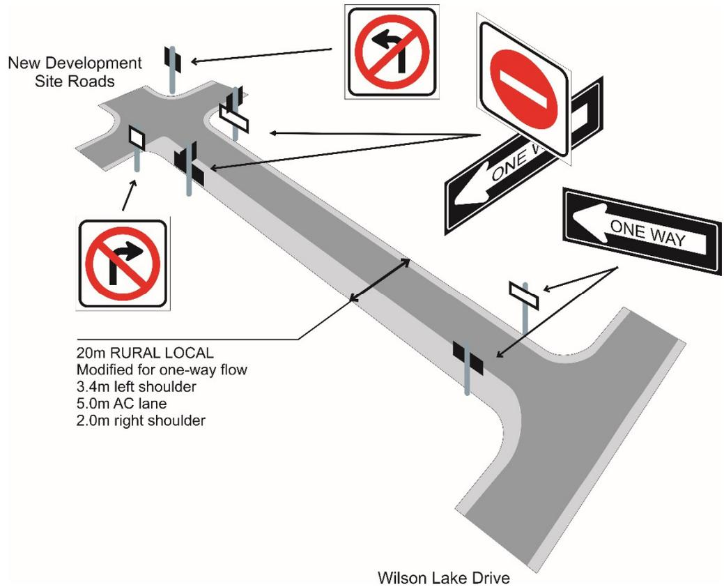
**Figure 3: Proposed Layout of One-way Connection to Wilson Lake Drive**
