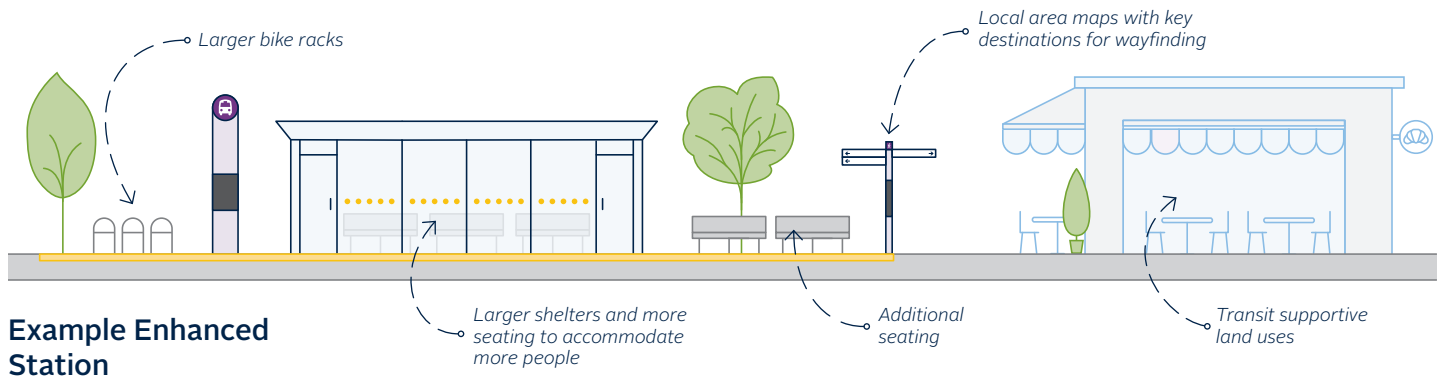
Figure 25: BRT enhanced station design example
