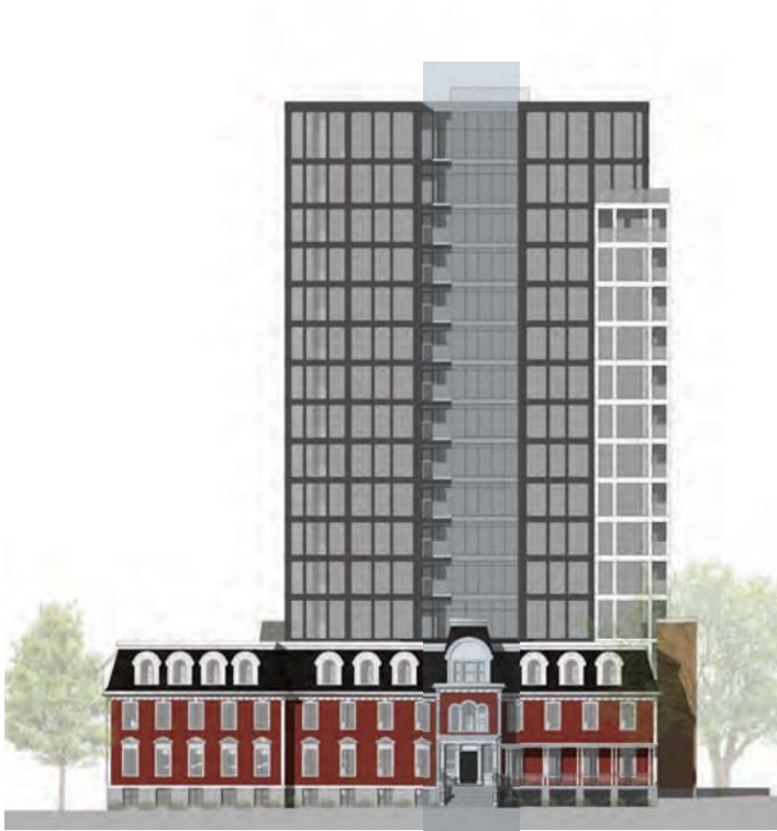
Fig. 28 Articulation and glazing on the East facade of the new building intentionally draws the eye to Victoria Hall's frontispiece
