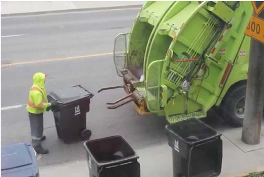
Figure D2: Semi-automated collection. Helper moves cart from the curb to a hydraulic tipper on the back of the truck. Cart is then returned to the curb.
