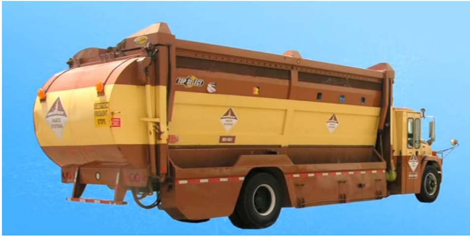
Figure D3: Side-loading recycling collection vehicle for manual collection. Compartments keep blue bags and paper recycling separate in the body of the truck.
