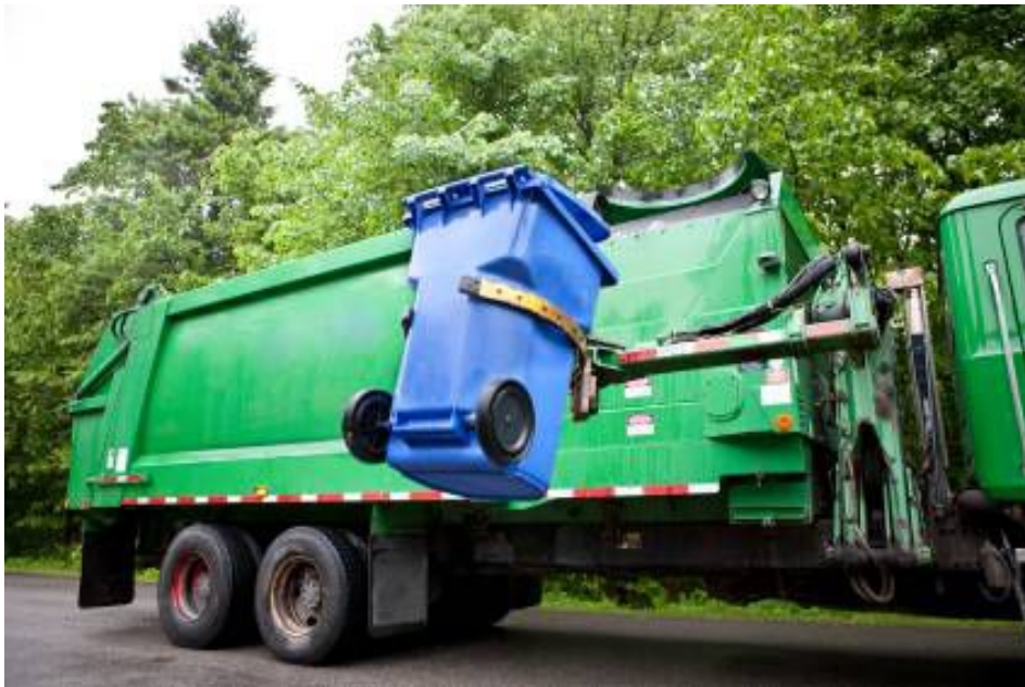
Figure D4: Fully-automated collection. Operator does not leave the cab of the truck. Controls an arm which picks the cart up and tips into the truck.
