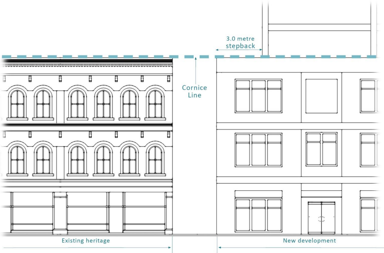
Diagram 15: Side wall stepback for taller portions of new detached buildings in a heritage context, as per Section 220
