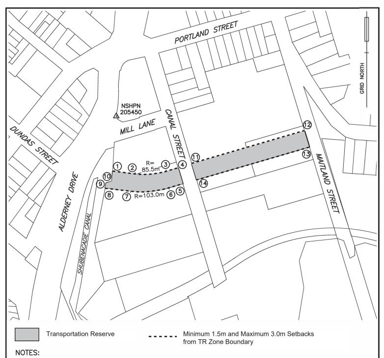
COORDINATES REFER TO ZONE 5, CENTRAL MERIDIAN 64°30' WEST, OF THE NOVA SCOTIA 3° MTM PROJECTION OF THE NAD83(CSRS) 2010.0 HORIZONTAL REFERENCE FRAME.
