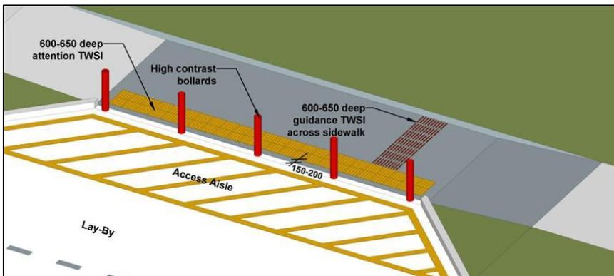
Figure 2: Accessible Loading Zone (Source: CNIB Clearing Our Path)
